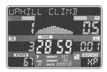
**Alpha Numeric Window:** The TR3000i and TR4000i come with a 16 character alpha window that is used to show the program name and other pertinent information during setup mode.
